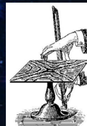
Creating a Chladni figure with a bow.
